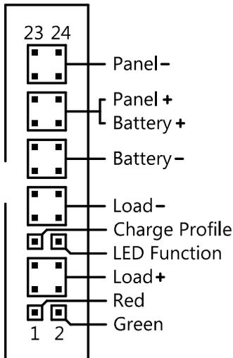
**Pin 1: Red LED Output.** Optional. Indicates errors. 56 Ohm output resistance, 15mA maximum source, 20mA maximum sink. See LED Function Select (Pin 8) description and LED Timings section for additional information.
