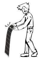
The panels should not be gripped by the ends and especially by the corners, to prevent them from flexing too much under their own weight.
