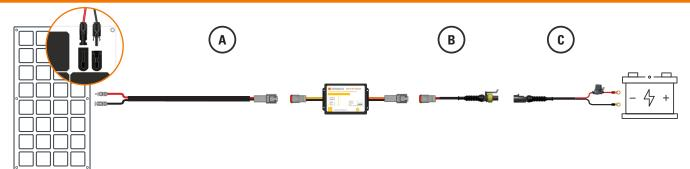
\*please make a drip loop! Water could run along the wires and cause water damage of the charge controller.
